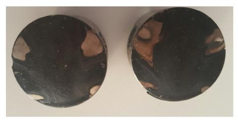
See pic on the Left for a set of pistons showing good piston wash, Piston wash (clear areas on a pistons surface) is created by the incoming unburnt fuel mixture cooling the piston surface as it enters via the transfer ports. The carbon deposits are only burnt on to the top of a piston where it is the
