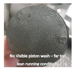
The second feature noticeable on a lean run is the underside of the piston surface (Remember "Black Spot Hot" – see pics below) when the piston temp is higher than it should be, the unburnt fuel from the crankcase will actually also burn a black spot onto the underside of the piston.
